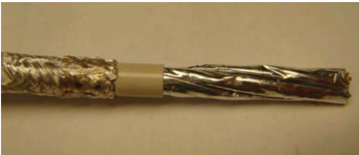
Figure 17: Sliding plastic bushing onto cable
