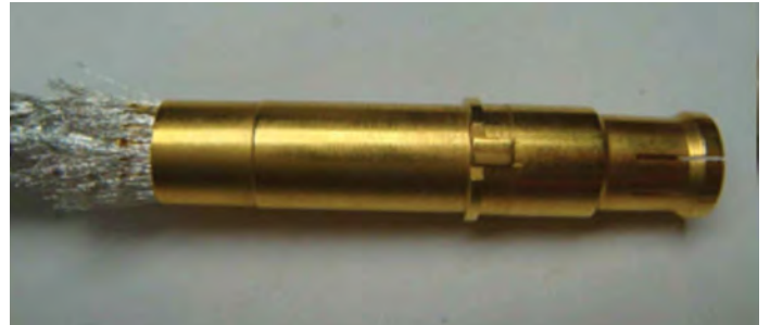
Figure 31: Installing outer body
