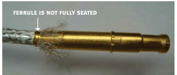
Figure 32: Pushing the ferrule
