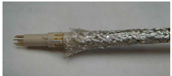
Figure 51: Returning the braid
