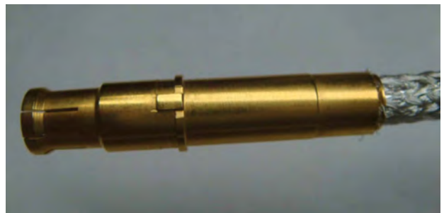
Figure 57: Trimming the braid
