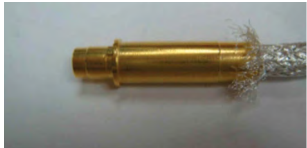
Figure 55: Installing outer body
