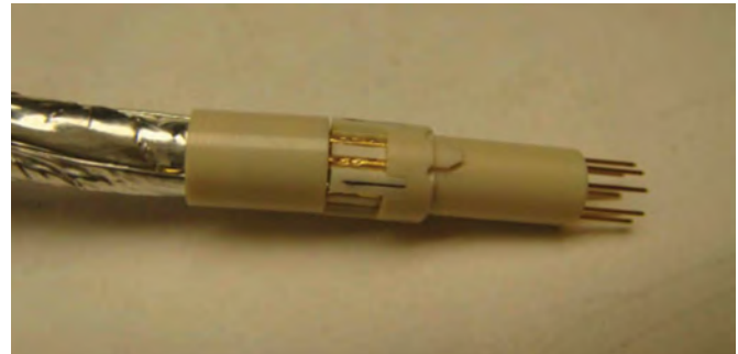
Figure 26: Returning the plastic bushing
