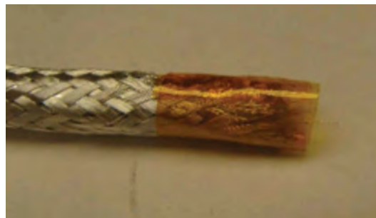
Figure 14: Taping the braid end
