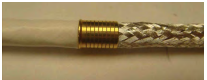
Figure 15: Sliding crimp ferrule on cable
