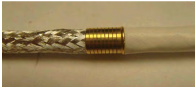
Figure 39: Sliding crimp ferrule on cable
