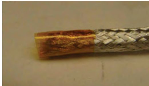
Figure 38: Taping the braid end
