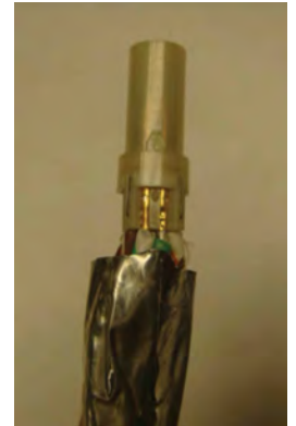
Figure 49: Seating the outer insulator
