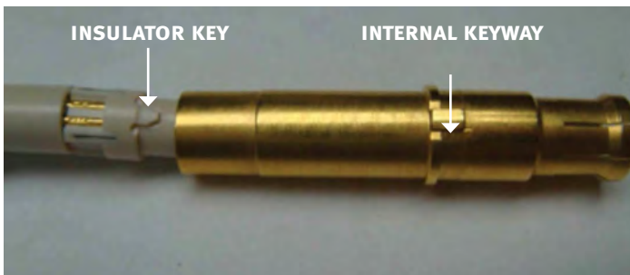
Figure 30: Aligning the keyway
