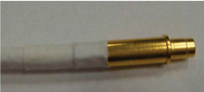
Figure 63: Shrinking tubing on crimp pin
