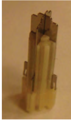
Figure 22: Inner insulator with metal spacers
