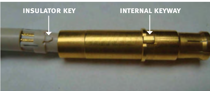
Figure 54: Aligning the keyway
