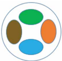
Figure 9: Pairs configuration at crimp socket end
