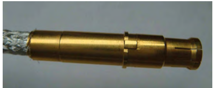
Figure 33: Trimming the braid
