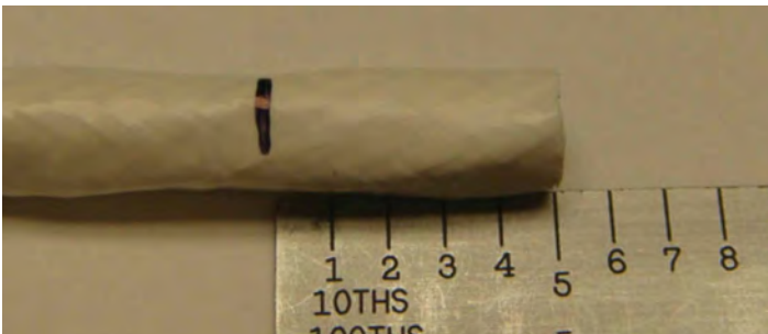
Figure 11: Marking the cable
