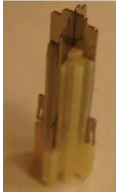
Figure 46: Inner insulator with metal spacers
