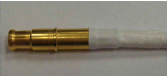
Figure 62: Shrinking tubing on crimp socket
