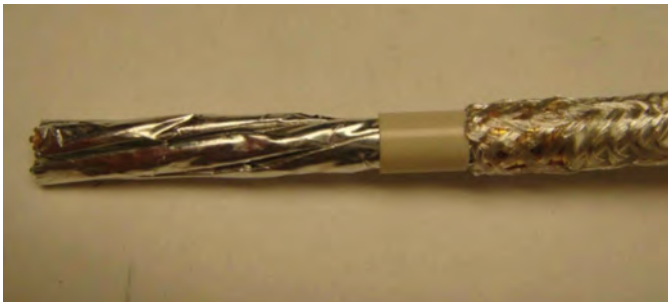
Figure 41: Sliding plastic bushing onto cable
